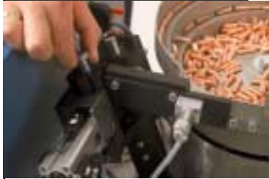
Quick-change system for conversion to other stud diameters (Patent No. DE 199 34 209 C2)
